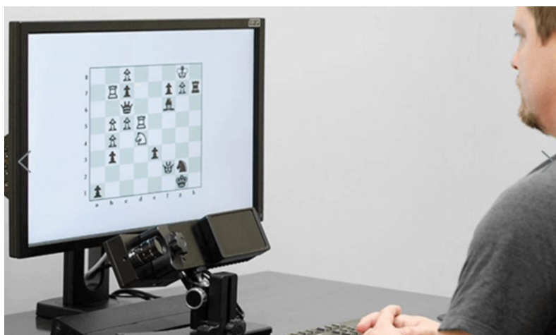
Figura 1: Rastreador ocular de desktop modelo Eyelink 1000 plus, fabricante SR Research. (Fonte: https://www.sr-research.com/eyelink-1000-plus/ )
